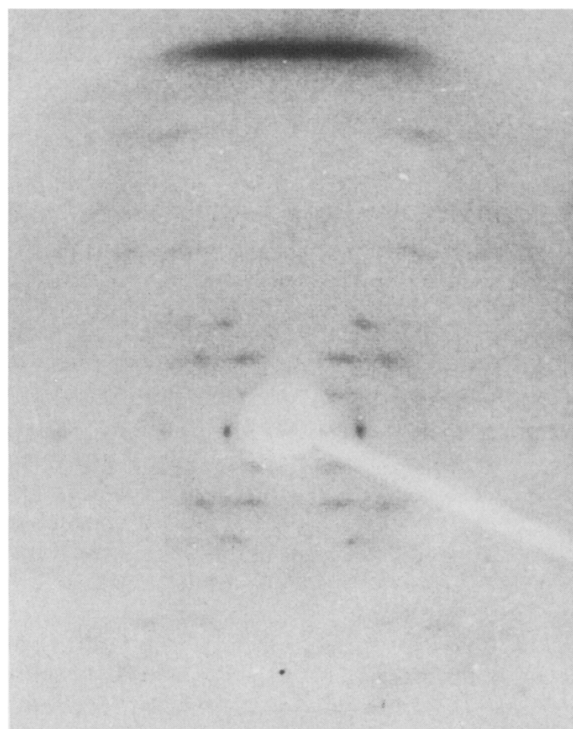
Fig.3. B-type diffraction patterns for Li-fibres appropriately tilted. The tenth layer meridional streak for (a, top) \Delta = 1.4 and (b, bottom) \Delta = 1.6 . Note the structure of this streak for the two salts: two off-meridional reflections for \Delta = 1.4 and a meridional and two off-meridional reflections for \Delta = 1.6 .
